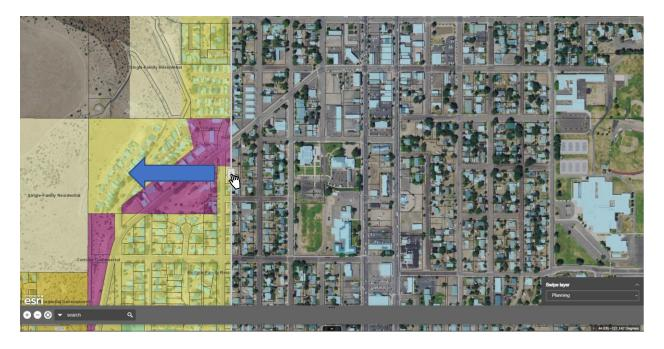
If multiple *data groups* are turned on, you can choose which one will be engaged by the *Swipe* widget by selecting a "Swipe layer" from the drop-down menu in the lower righthand corner of the map view.
