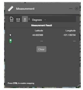
With the Location button selected, the choice for units are Decimal Degrees and DMS (Degrees, Minutes, Seconds). These can be found in the drop-down menu on the right.
