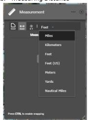
With the measure distance button selected, the options for measurement units can then be viewed and selected using the drop-down menu on the right.
